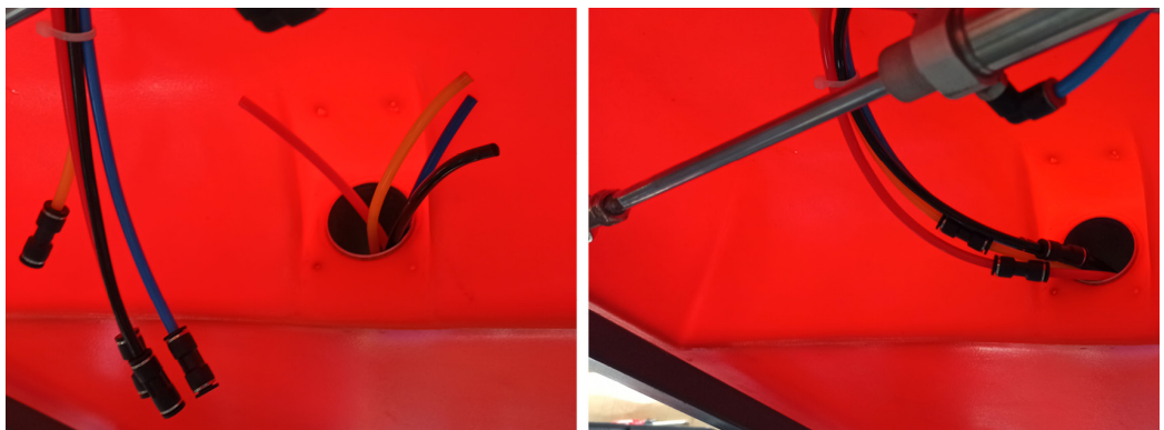
Figure 18. Attaching air lines.
