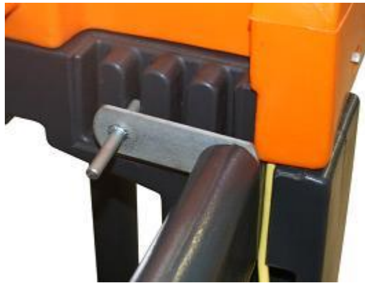
Figure 8. Slots and locking lever to allow Sheep Auto Drafter width adjustment.
