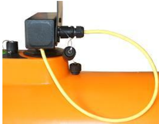
Figure 19. The loop back cable.
