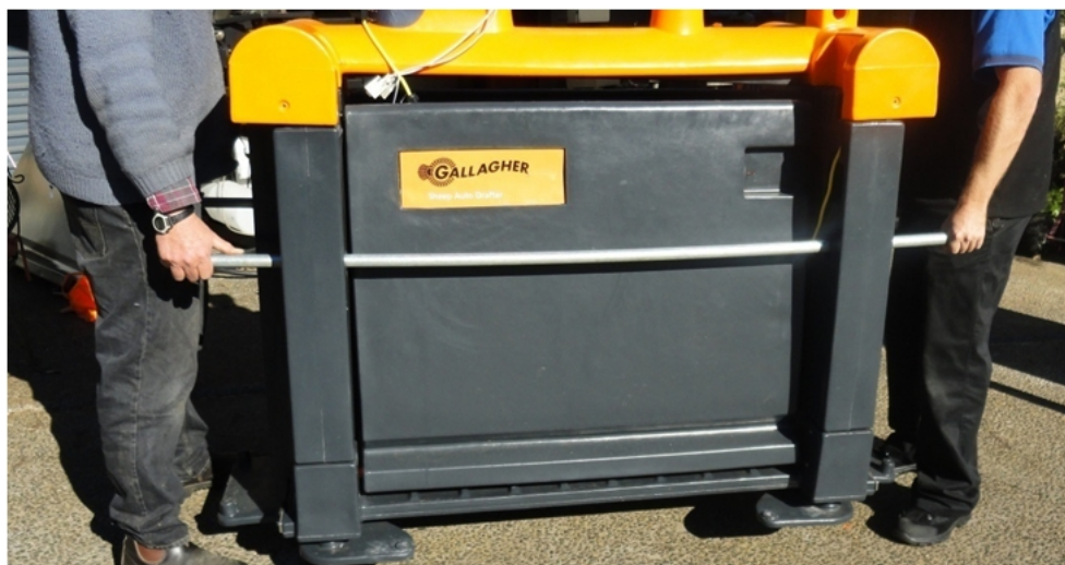
Figure 5. Lifting using the transport poles.
